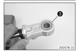
Remove seal rings 3 on both sides.
