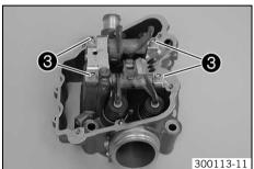
Install and tighten the screws 3 of the rocker arm shafts.
