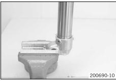
Release the fork leg and clamp it with the fork stub.
