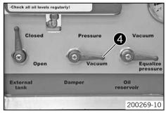
When the pressure gauge reaches the specified value, turn the Damper 4 control lever to Vacuum.
