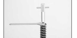
Pull the spring downward. Mount the special tool on the hexagon.
