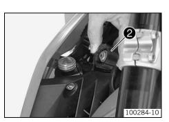
Correct the coolant level and find out the cause of the loss.
