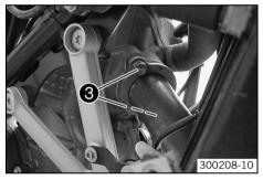
Remove nuts 3 of the manifold.
