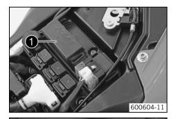
Remove the defective fuse.
