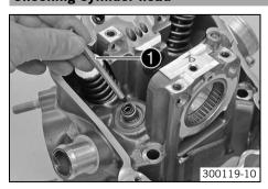
Check the valve guides using the special tool **1**.
