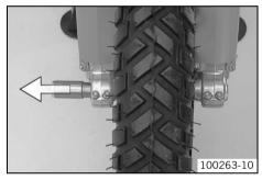
Holding the front wheel, withdraw the wheel spindle. Take the front wheel out of the fork.
