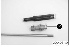
Take screw sleeve ② off of the cartridge along with the washer and spring seat.
