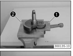
Removing crankshaft bearing inner ring
