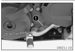
The engine number  ${\ensuremath{\bullet}}$  is stamped on the left side of the engine under the engine sprocket.
