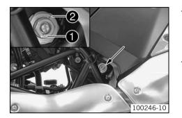
Turn adjusting screw **1** all the way clockwise using a socket wrench.
