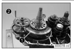
Remove the crankshaft ① and the balancer shaft ②.
