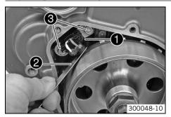
Adjust the distance between the crankshaft position sensor ① and the conductive element of the rotor using the special tool ②.
