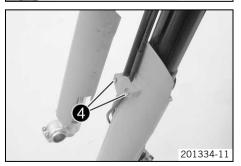
Slide on the fork protector from above and position it. Mount and tighten screws **1**. Guideline
