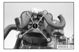
Put the valve cover in place with the seal. Mount and tighten screws ①.
