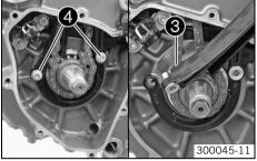
Position the timing chain securing guide  $\mathbf{0}$ .
