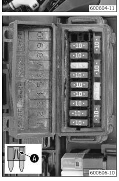
Remove the defective fuse.
