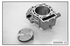
Use the special tool to measure clearance I of the piston rings in the piston ring groove.
