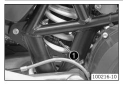
The shock absorber part number **1** is on the right of the shock absorber.
