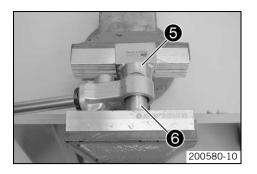
Place special tool <sup>(6)</sup> underneath and press out the heim joint with special tool <sup>(6)</sup>.
