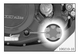
Check the engine oil level.
