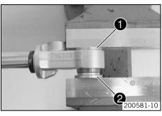
Place special tool ① underneath and press in the heim joint as far as the center using special tool ②.
