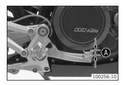
Move the foot brake lever back and forth between the end stop and the contact to the foot brake cylinder piston and check free travel (). Guideline
