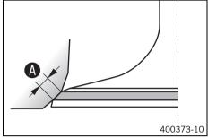
Check the sealing area of the cylinder for distortion using a straight edge and the special tool.
