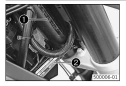
The chassis number ① is stamped on the right of the steering head. The type label ② is on the right of the frame behind the steering head.
