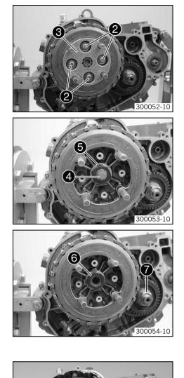
Loosen the screws ② diagonally and remove them with their spring retainers and clutch springs.
