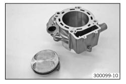
Nikasil<sup>®</sup> is a surface protection layer for a coating method developed by the Mahle company. The name is derived from the two materials used in this method - a layer of nickel, in which silicon carbide (a particularly hard substance) is embedded. The most important advantages of the Nikasil<sup>®</sup> coating are the excellent heat conductivity resulting in better performance, less wear, and low cylinder weight.
