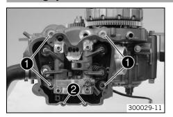
Put on the cylinder head gasket.
