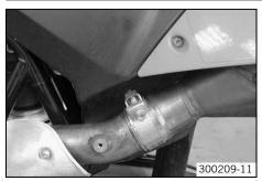
Position the manifold at the rear with the seals. \_
