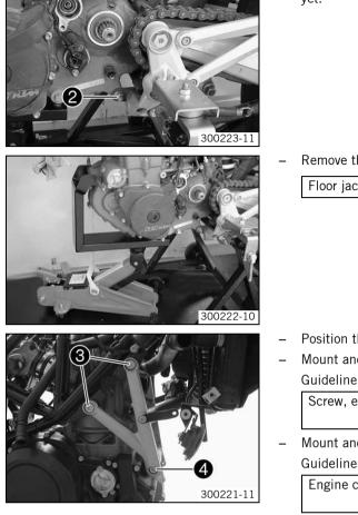
Install the screw and nut **2** of the lower engine bracket, but do not tighten them yet.
