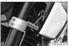
The Canada type label **③** is on the right of the frame behind the steering head.
