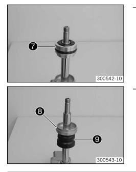
Remove seal ring retainer 🕖.
