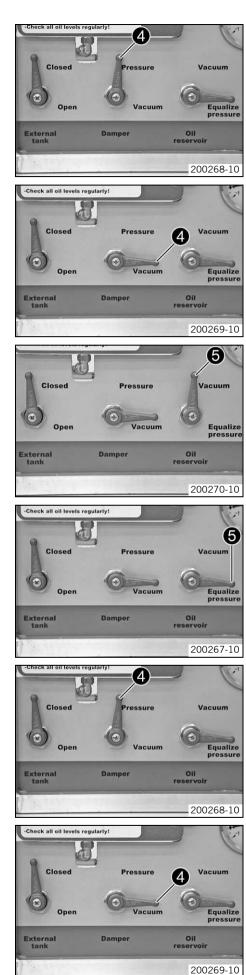
When the pressure gauge reaches the specified value, turn the **Damper** control lever **4** to **Pressure**.
