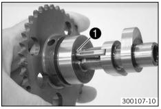
Take the lock ring **1** off the autodecompression shaft and dispose of it.
