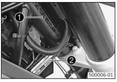
The chassis number **1** is stamped on the right of the steering head. The USA type label **2** is on the right of the frame behind the steering head.
