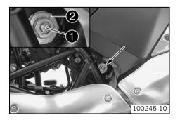
Turn the adjusting screw  ${\ensuremath{\bullet}}$  clockwise with a screwdriver up to the last perceptible click.
