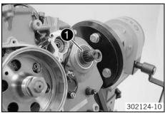
Grease the shaft seal ring.
