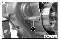
Set the crankshaft to top dead center and lock it with the special tool  $oldsymbol{0}$  .
