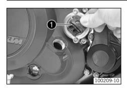
Remove the oil filler plug with O-ring **1** from the clutch cover and fill up with engine oil.
