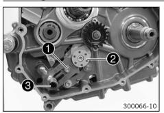
Push sliding plate 1 away from the shift drum locating 2. Remove shift shaft 3 with the washer.
