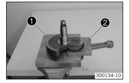
Fix the crankshaft with special tools **1** and **2** in the vise. \_
