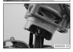
Cover the engine case opening with a cloth. Thread the timing chain through the chain shaft. Mount the piston pin.
