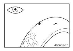
Check the front and rear tires for cuts, run-in objects and other damage.
