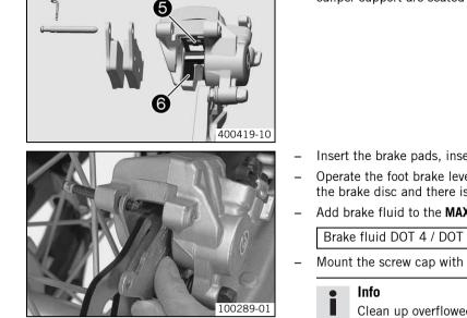
Check that leaf spring **③** in the brake caliper and sliding plate **③** in the brake caliper support are seated correctly.
