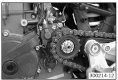
Reconnect plug connectors I of the gear position sensor, the crankshaft position sensor and the alternator.
