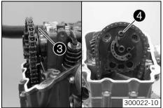
Lay the timing chain over the camshaft. Push the timing chain into the bearing seats. The middle drill hole of the camshaft ● and the drill hole of the cylinder head ② must be aligned.
