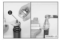
Pull the spring downward. Mount the special tool on the hexagon.
