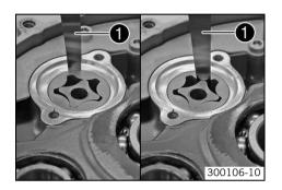
Use a feeler gauge **1** to measure the play between the external rotor and the engine case as well as between the external rotor and the internal rotor.
