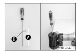
Slide O-ring <sup>(3)</sup> to the end of the special tool by the specified value (distance <sup>(3)</sup> minus specified value).
