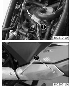
Remove the air filter box. (\* p. 63) Unplug connector **1** of the lambda sensor. Open the cable binder. \_
