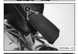
Position the splash protector. Mount and tighten screws 4.
