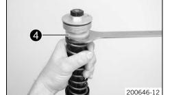
Preload spacers 4 should be above the special tool.
