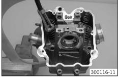
Pretension the valve springs using the special tool.
