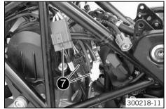
Reconnect plug-in connections of the gear position sensor, the crankshaft position sensor and the alternator.
