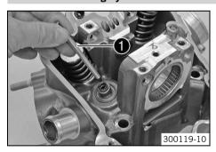
Check the valve guides using the special tool **①**.
