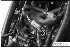
Plug in the connector of the lambda sensor 3. Secure the cable with the cable binders.
