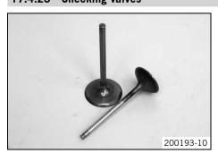
Check the run-out at the valve plate.
