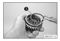
Insert the lock ring (a) into the groove with suitable pliers and check that it is seated correctly.
