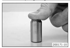
Fully compress the timing chain tensioner.
