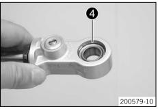
Remove lock rings 4 on both sides.
