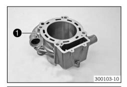
Check the sealing area of the cylinder head for distortion using a straight edge and the special tool.
