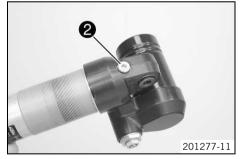
Clamp the damper in the vise using soft jaws.Fill the damper cartridge about half full.
