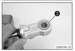
Remove seal rings 3 on both sides.
