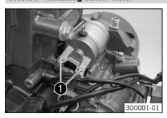
Grease O-ring. Mount the starter motor.
