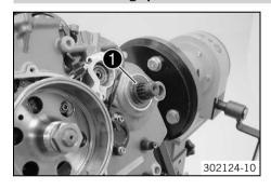
Remove the spacer • of the countershaft.
