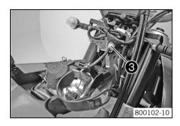
Disconnect the electrical plug-in connection 3 and remove the headlight mask with the headlight.
