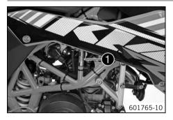
The type label  $\bullet$  is located on the right side of the frame.
