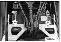
Stator winding - check for a short circuit to ground (terminal 31)
