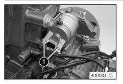
Remove screws **①**. Take off the starter motor.
