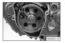
– Mount the tab washer and the nut **2**. Tighten nut.
