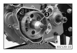
17.3.20 Removing timing chain rails
