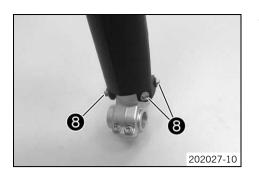
Remove screws ③. Remove the fork protector from above.
