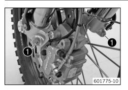
Turn adjusting screws  $\ensuremath{\bullet}$  clockwise all the way.
