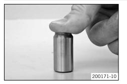
Fully compress the timing chain tensioner.
