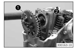
Lay the timing chain over the camshaft. Push the timing chain into the bearing \_ seats. The middle drill hole of the camshaft 1 and the drill hole of the cylinder head **2** must be aligned.
