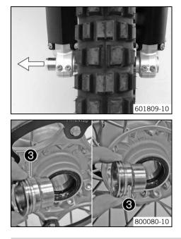
Holding the front wheel, withdraw the wheel spindle. Take the front wheel out of the fork.
