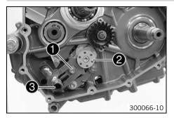
Push sliding plate ① away from the shift drum locating ②. Remove shift shaft ③ with the washer.
