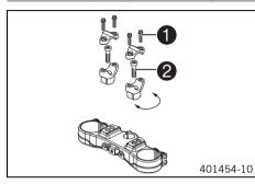
Remove the four screws **1**. Remove the handlebar clamp. Remove the handlebar and lay it to one side.
