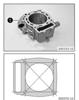
The cylinder size  $\mathbf{0}$  is marked on the side of the cylinder.
