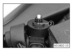
Turn the adjusting wheel until the desired digit is next to marking ②.
