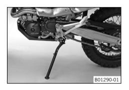
Remove the motorcycle from the lift stand and rest it on its side stand.
