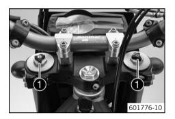
Turn adjusting screws ① clockwise all the way.
