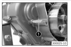
Set the crankshaft to top dead center and lock it with the special tool  $oldsymbol{0}$ .
