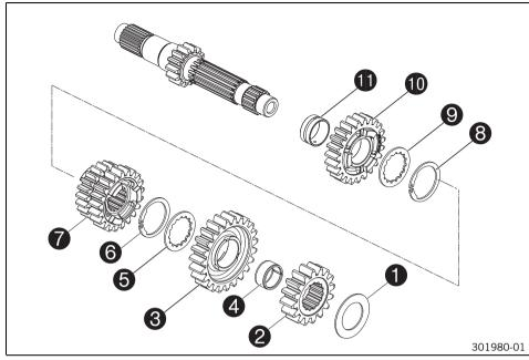
Fix the main shaft in the vise with the geared end facing downward. Guideline
