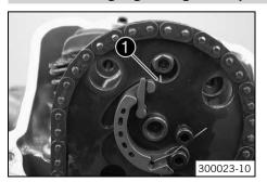
Turn the crankshaft counterclockwise until markings **1** of the camshafts are flush with the marks of the camshaft support plate.
