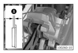
Check the brake linings for minimum thickness **(**).
