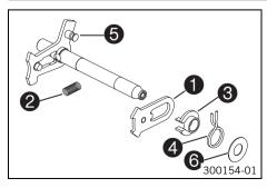
Fix the short end of the shift shaft in a vise.
