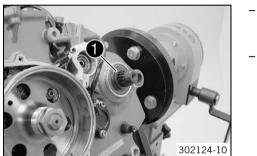
Grease the shaft seal ring.
