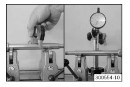
Measure the diameter of the piston rod.
