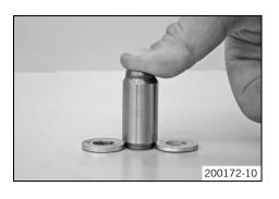
Place two compensating disks or similar aids next to the piston of the timing chain tensioner. This should ensure that when pushed down, the piston does not fully withdraw.
