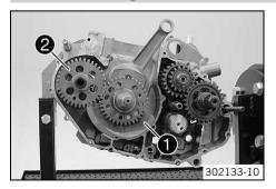
Remove the crankshaft **1** and the balancer shaft **2**.
