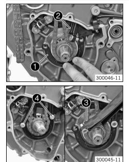
Position the timing chain securing guide ①.
