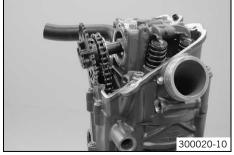
Remove screw **①**. Take off the camshaft support plate **②**.
