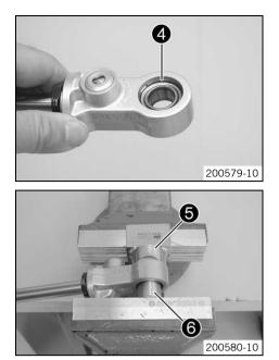
Remove lock rings ④ on both sides.
