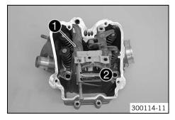
Position the rocker arm **1** and push in the rocker arm shafts **2**.
