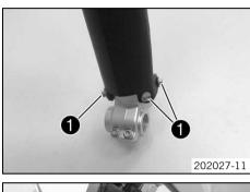
Slide on the fork protector from above and position it. Mount and tighten screws ①.
