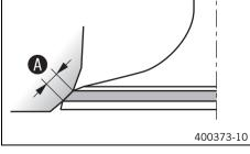
Check the run-out at the valve plate. \_
