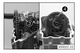
17.5.20 Installing timing chain tensioner
