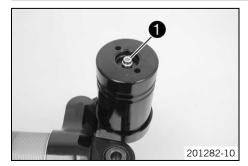
Screw in screw **1** by approx. 2 rotations but do not tighten.
