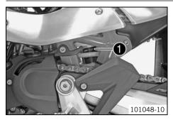
The shock absorber part number **1** is on the left of the shock absorber.
