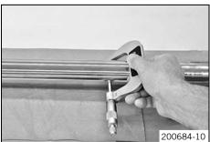
Measure the external diameter of the inner tube in several places. \_
