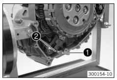
Remove the spacer ① and spring ② of the shift shaft.
