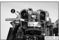
Check the valve clearance on all valves between the valve and the rocker arm using the special tool ②.
