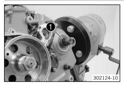
17.3.7 Removing gear position sensor
