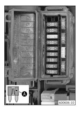
Remove the defective fuse.
