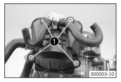
Put the valve cover in place with the seal. Mount and tighten screws **1**. \_ Guideline
